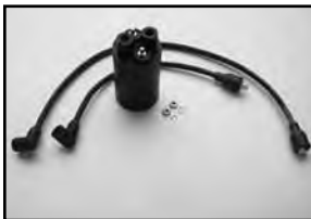
Ignition Coil (Battery)
