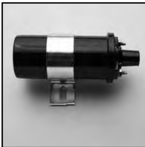
Ignition Coil (Battery)
